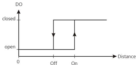
The ON level of the hysteresis is larger than the OFF level. With an increasing distance, the digital output is switched on (open drain output is closed) when the distance exceeds the ON level. With a decreasing distance, the digital output is switched off (open drain output is open) when the distance falls below the OFF level.
