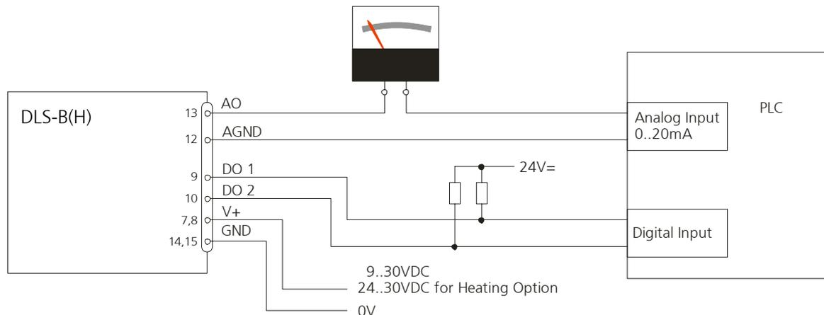
Fig. 6 Connection of an instrument and a PLC
