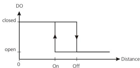
The ON level of the hysteresis is smaller than the OFF level. With a decreasing distance, the digital output is switched on (open drain output is closed) when the distance falls below the ON level. With an increasing distance, the digital output is switched off (open drain output is open) when the distance exceeds the OFF level.
